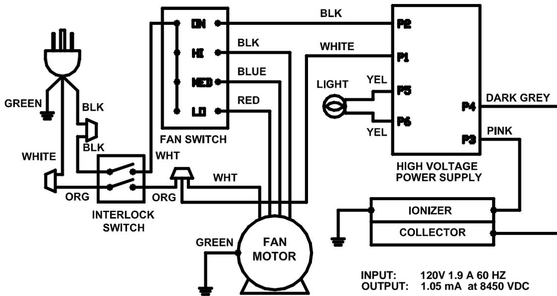
FIGURE 6 – 120V SCHEMATIC
