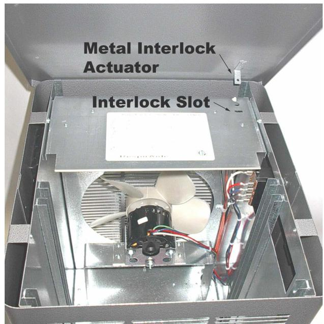
**FIGURE 4 – THE COVER MUST FIT CORRECTLY FOR OPERATION. IONIZER WIRE REPLACEMENT**
